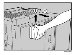
2 Remove the dustproof filter slowly by holding the tab on the bottom, and then put it in the bag that the new filter came in.
