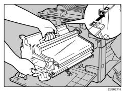
By holding the beige handle of the photoconductor unit as shown in the illustration, tighten the screw that you released in step
