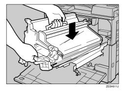
Set the photoconductor unit by placing it on the guide with a label (△). Matching the arrow on the unit and the label makes it easy to place the unit on the guide.
