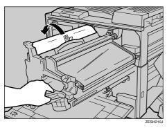
By holding the beige handle of the photoconductor unit, insert the unit slowly until it stops.
