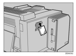
4 Set the dustproof filter cover that you removed in step ●. Insert the projections in the holes (①), and then push downwards (②).
